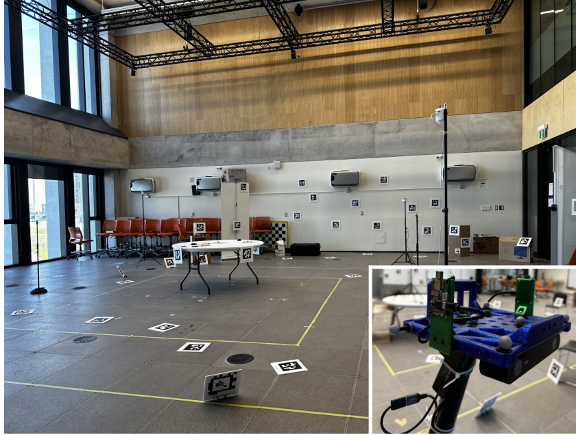
Fig. 1. The STAR-loc dataset contains data collected on different trajectories of a sensor rig (bottom right) in a Vicon mocap arena, providing range and calibrated stereo measurements.
