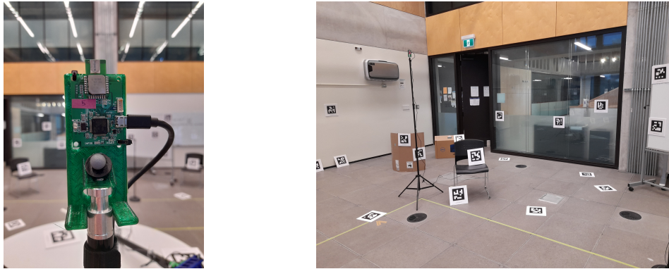
Fig. 3. Left: One of eight fixed UWB anchors. Right: subset of Apriltag landmarks.
