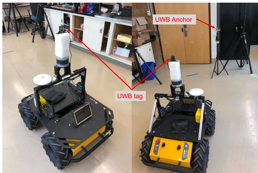
Figure A.4: The experimental set-up with one tag on a robot rotating in place and another tag on a static tripod.
