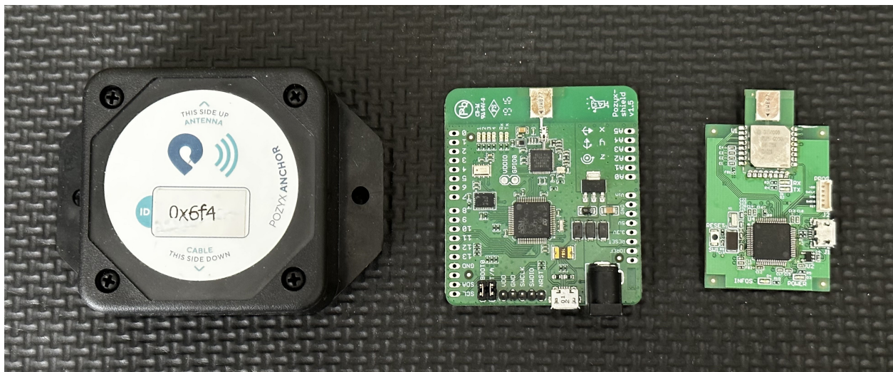
Figure A.1: The different UWB transceivers used. (Left) Pozyx anchor. (Middle) Pozyx tag. (Right) Custom-built tag.
