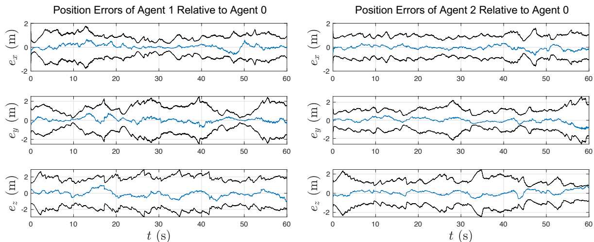
Figure 3.10: The performance of the relative position estimator on experimental data for both the two-tag Agent 1 and the single-tag Agent 2, where the black lines represent the \pm 3\sigma bound of the estimator.
